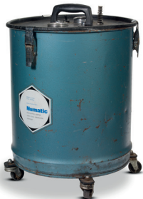
First Numatic vacuum cleaner, engineered for cleaning coal, oil and gas fired boilers
